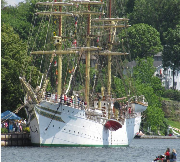
Sørlandet was built of steel in 1927 at Høivolds Mek. Verksted in Kristiansand, to be used as a school ship for the Norwegian Merchant Marine. She is a three-masted full-rigged ship carrying royals over single topgallant sails. Originally built without power, an engine and propeller were installed in 1958. She is now the oldest and best kept full-rigged ship in operation.
